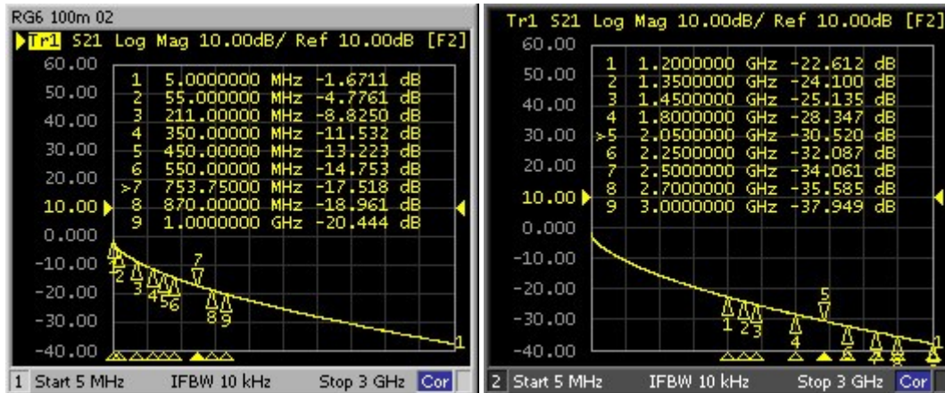
Insertion loss of Tri-Shield DIPOLNET RG-6 Cu cable as a function of frequency (5-3000 MHz)
